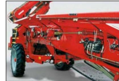
*Intelligent construction: All hydraulic and electronic components located within the supporting side frame: protected from soil and damage*
