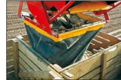
Without deflection from the target: the optional box filling chute with easy attachment to the cart elevator head. For trouble-free filling directly into potato boxes or as a fall breaker into tall trailers
