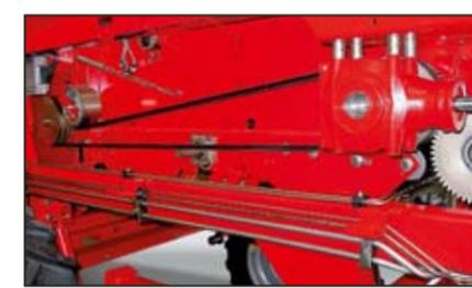
*Innovative. Long lasting. Efficient. The drive construction benefits from the use of tough angular gearboxes and low maintenance v-belt drives.*
