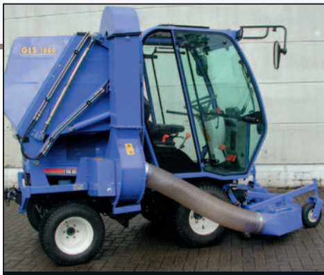
SF310 with optional cab and side collection blower
