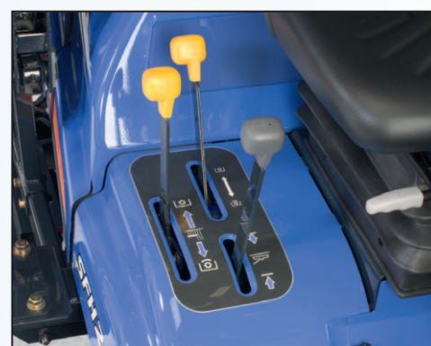
Levers fall readily to hand for deck lift/lower, PTO to blades and blower
