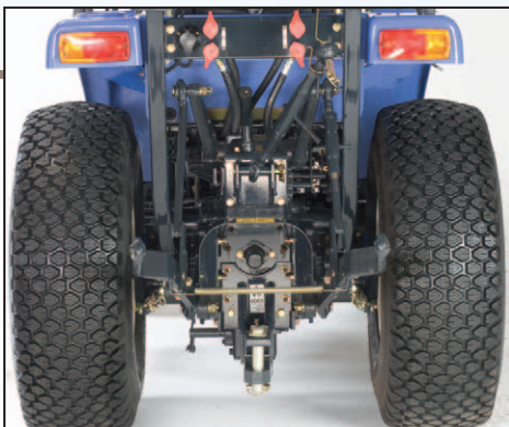
Category 1 3-point linkage with 1100 kg lifting capacity
