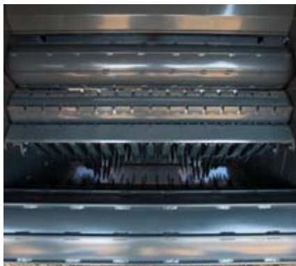
The bale chamber concept consists of 5 rollers at the front...
