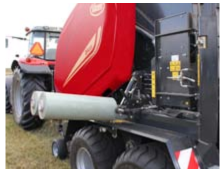
Stretch film cassette with hydraulic operation for maximum operator convenience.
