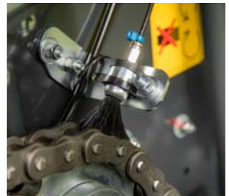
Automatic chain lubrication is standard on RF4225
