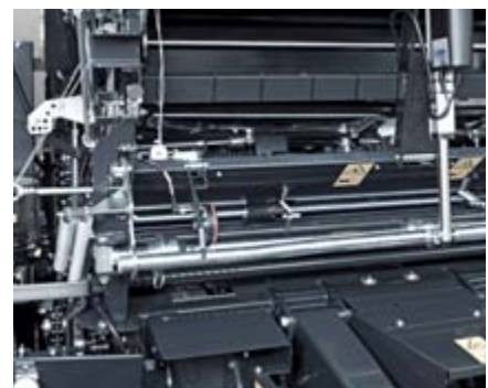
Twin tube fast operating twine binding system.
