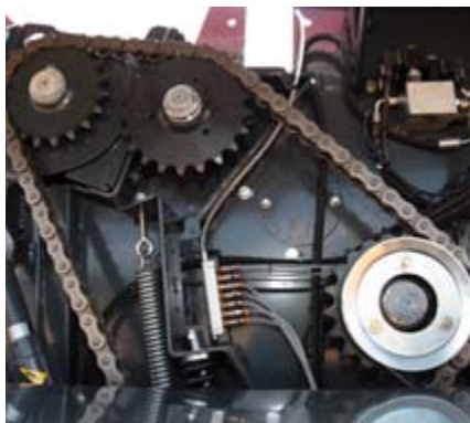
Main bale chamber drives are by heavy duty 1 1/4" pitch chain for a longer lifetime and reduced maintenance
