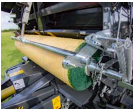
New high efficiency PowerBind net wrap system.
