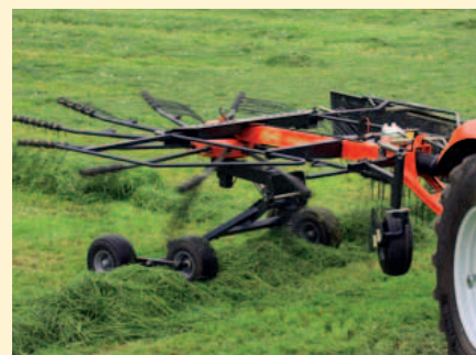
The machine can conveniently be raised up to a height of 50cm from the tractor driver's seat.
