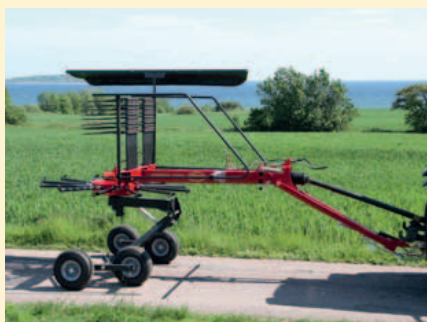
With a linkage mounted drawbar, the Index 474T can be easily operated by low horse power tractors.
