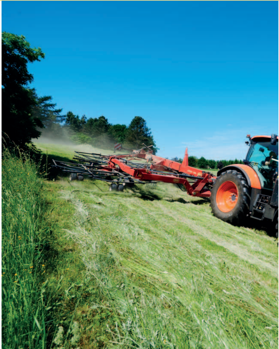
The unique elbow construction positions the front rotors close to the driver for excellent overview.
