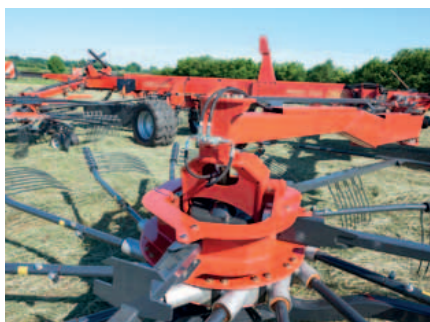
Each rotor can be independently set for height using the hydraulic system.
