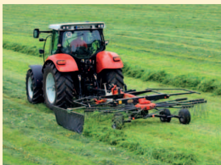
Index 474T – 4.70m working width and a weight of only 665kg.
