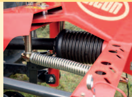
A pivoting 3-pt headstock ensures perfect ground following performance, and perfect tracking when cornering. Oscillation dampers are optionally available.
