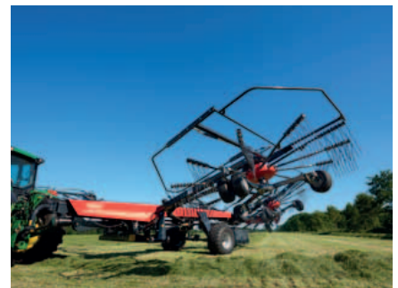
High lift of rotors ensures generous clearance during headland turns.
