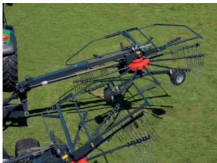
Working width can be set hydraulically between 10-12.5m. Swath width is also set hydraulically between 1.2 and 2.2m.
