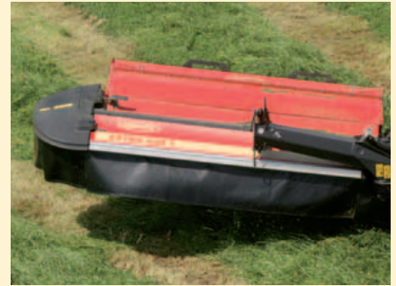
Easy lift on headlands without activating the 3pt linkage of the tractor.
