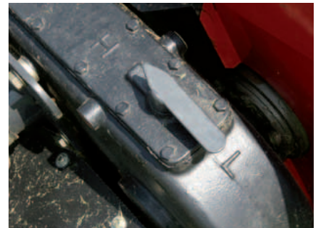
Conditioner speed of 900 or 600rpm - changed in a second.
