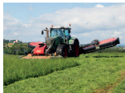
Automatic headland control – front mower is lowered before the rear mowing units.
