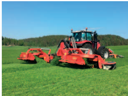
With the Vicon swath belt, grass from either 6.00m or 9.00m can be placed in a single swath.
