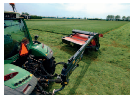
The swivel hitch headstock with reversible gearbox provides optimal manoeuvring ability.
