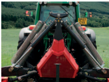
4 large springs ensure even flotation and cutting height.
