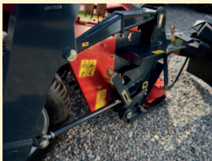
The special suspension rod ensures that the mowing section is automatically lifted upwards and above the object.
