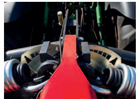
Large suspension springs, optionally with hydraulic setting of ground pressure.
