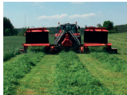
When not in use the optional Vicon swath belt is raised hydraulically to a position above the mowing units.
