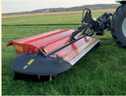
Pulled centre suspension for even weight distribution and excellent adaptation.
