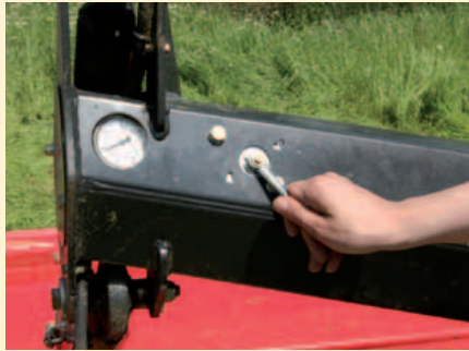
Hydraulic suspension for easy and precise setting of ground pressure.
