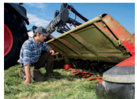
Easy and quick access to the cutterbar for daily inspection of discs and blades.
