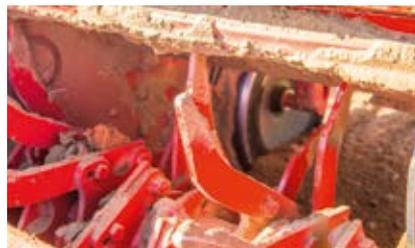
Hard metal tines (2) have a highly wear-resistant coating, so-called widia plates, that are vacuum-soldered. They are not suitable for stony conditions.
