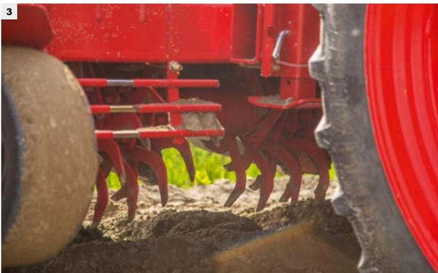
Spikes (4) are especially designed for soils with high content of stones and stones up to fist-size (> 5 cm). The spikes are easy to replace, because they are fastened by a single screw.
