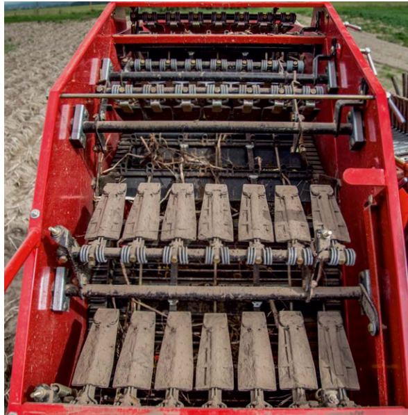
Optimal crop protection: deviner web with soft PU flights (distance each 210 mm)
