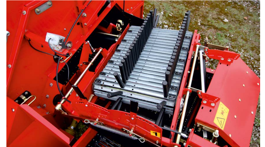
Infinitely hydraulic speed adjustment of the finger web.
