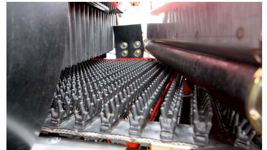
The roller scraper ensures a loss-free separation of potatoes and trash.
