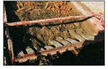
Clod breaker (option) Breaking through. An option for very cloddy soils
