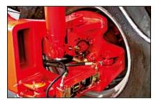
Hydrostatic wheel drive (option) Easier harvesting – even in heavy conditions: with the hydrostatic wheel drive
