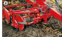
Hydraulic drawbar adjustment (option) Digging on the right track: the hydraulic drawbar (1) adjustment keeps the GT170 in line, even on hillsides.
