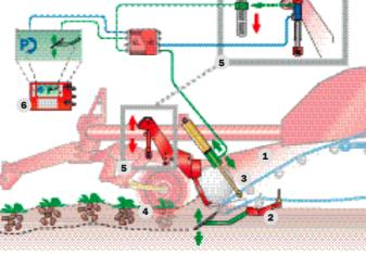
have integrated linear measuring and pressure reading systems. Each cylinder reads every variation to the ridge height and sends an electronic signal to the left or right cylinders which control the swinging frame. The result: the digging depth remains the same all the time, irrespective of how uneven the ground is – and is even independent for each row!
