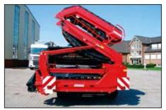
Ready for the road: For road transport the cart elevator folds hydraulically to a compact position.
