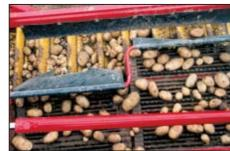
Reversing: cart elevator reversing kit with delivery chute for windrowing between adjoining rows
