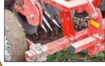
Carrot intake (option) The robust carrot share works with large, distance adjustable support wheels and a manual depth adjustment. Various row distances available on request
