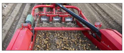
The look into the new dimension: 3-row digging with the GT 300 (5). The proven straight-lined harvest flow and the slight incline of the main webs make this machine very gentle to the crop and ensure high performing.
