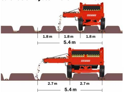
The MAXI-Bed places proven system steps onto a new, wide basis. Machines widths are aligned during bed forming, via separating (1) and planting (2) all the way to the harvest. They provide 50% more surface yield during each work sequence.
