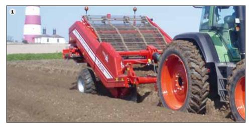
CS 240 (1): Sieve the stones and crush the clods: This gives an evenly aerated bed and will provide optimal growth conditions for potatoes and other vegetables – and this in a whole new width.
