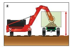
Reverse: With the optional function of windrowing, the cart elevator can be reversed. I.e. the deposit funnel ensures the swath deposit between the two adjacent rows (3).
