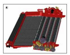
More success with the double pack: Combine the MULTISEP (3) or the Roller separator (4) with an additional MULTISEP. The separator units can be operated separately in their feeding and cleaning performance; therefore, they can react optimally to changing conditions.
