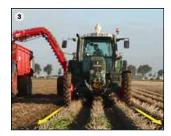
Harvesting with the offset system: the tractor drives over 2 instead of 3 rows (2), the GT 300 continues offset behind the tractor and therefore harvests an additional row to the left of the tractor.
