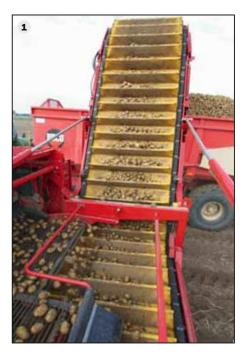
A very gentle feeding. Highest possible flexibility. And 160 t/h feed performance! – This makes the cart elevator of the GT 300 so special. The active lateral parts as well as the length and flexibility of the elevator ensure a smooth and gentle feeding of the harvest stream.
