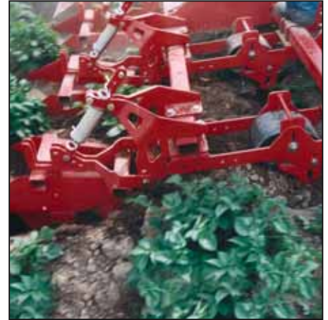
Loose soil: the individual row shaper at work
