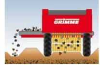
Phase 2: Bed separation with the stone and clod separator of the CS-Series. The separator takes up the entire bed width and sieves the soil.
