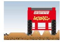
Phase 3: Potato planting with the bed planting system. Immediately after separation, the seed potatoes are planted using the 1-, 2- or 3-bed system
