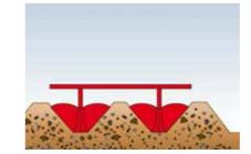
Phase 1: Bed formers of the BF/BFL-Series shape the beds. The track and bed widths are determined during this step.
