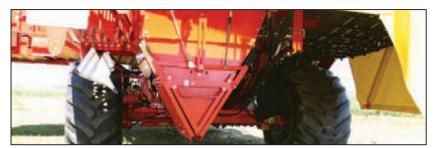
Small hopper under the pre-grading unit (option)
