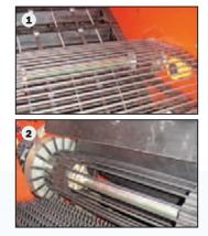
Minimum drop stages, gentlest crop handling: thanks to the reduction of the drop size from the 1st to the 2<sup>nd</sup> main web (1). This is made possible by an almost horizontal feed. The very small drop from the 2<sup>nd</sup> main web onto the  $1^{st}$  separator (2) is gentle on the crop. - Like the web bars, which in addition clean the walls of the side panels.
