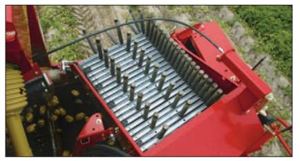
The speed of the finger web is infinitely hydraulically adjusted.
