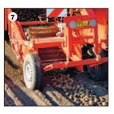
Windrow intake with share blades: consisting of support wheels, hydraulic depth adjustment and adjustable brush web speed especially suited for very light soil types.
