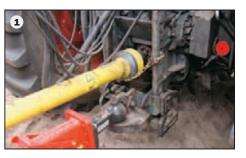
As an alternative, the machine is secured attached underneath the PTO connection. All eyelets can be height adjusted (1) to fit different tractors.
