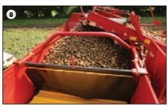
The optional stone box (6) has a capacity of approx. 500 kg. The filling process takes place via favourably positioned easy pick chutes; the emptying takes place manually via a foot pedal at the picking stand. Hydraulic emptying from the tractor cab is available as an option.
