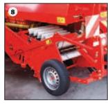
Windrow-intake via rotor shaft: consisting of rotor shaft for minimum soil intake, support wheels, hydraulic depth adjustment as well as adjustable brush web speed.
