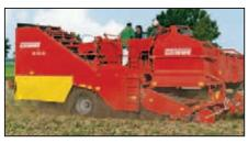
SE 150/170-60: 2-row, offset trailed potato harvester, gentle, efficient and reliable harvesting, with large bunker for 6,000, 7,000 or 7,500 kg
