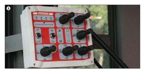
From hands-on use to hands-on use: The offset intake on the right-hand driver's side corresponds to the ergonomics of the driver's cabin and makes for easy machine handling. All important machine functions as well as the optional hydraulic share depth adjustment and ridge relief can be comfortably controlled from the driver's seat (1).
