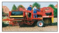
SE 75-20: 1-row, for small to medium-sized fields, special compact (low) design, moving floor bunker for 2,000 or 2,300 kg
