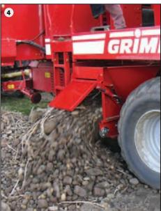
4 grading rollers (1) reliably separate smaller sizes. The roller spacing between 0 and 40 mm can be infinitely adjusted via a central control. A roller speed increasing with the direction of flow protects the crop.
