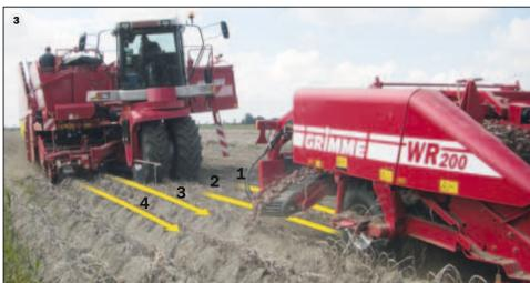
2+2=4: The economical alternative to the 4-row harvester. The WR 200 in its enriched process. The potatoes are picked up by a 2-row potato harvester (3).
