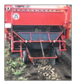
The WR 200 with its long main web deposits the potatoes into a swath featuring a width of approx. 130 cm (1). Afterwards, they are picked up by hand.
