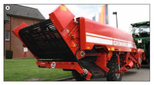
The fine haulm elevator (4) on the WR 200 for increased haulm separation.
