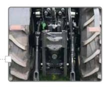
More flexibility with hydraulic stabiliser struts easily controlled from inside the cab.
