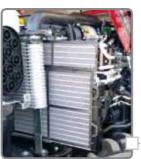
Quantum engines are equipped with turbocharger and an air to air intercooler to boost thermal efficiency and extract maximum power from every drop of fuel.
