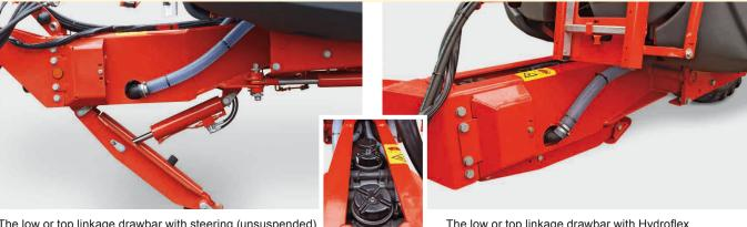
The low or top linkage drawbar with steering (unsuspended) allows short turning on the headland. Pumps are well protected and integrated in the drawbar.
