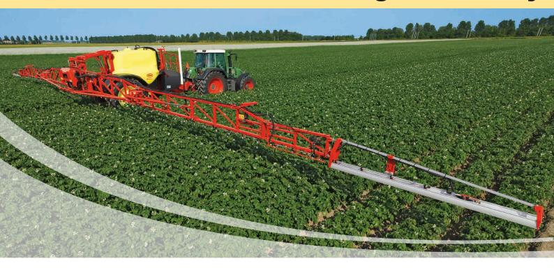
Perfect boom guiding in hilly or flatland position through a professional double trapezium balancing system. In flatland position the boom is perfectly levelled out and compensates a wrong position of the sprayer compared to the field shape. In hilly conditions the HBWP boom is following automatically the inclination of the sprayer.
