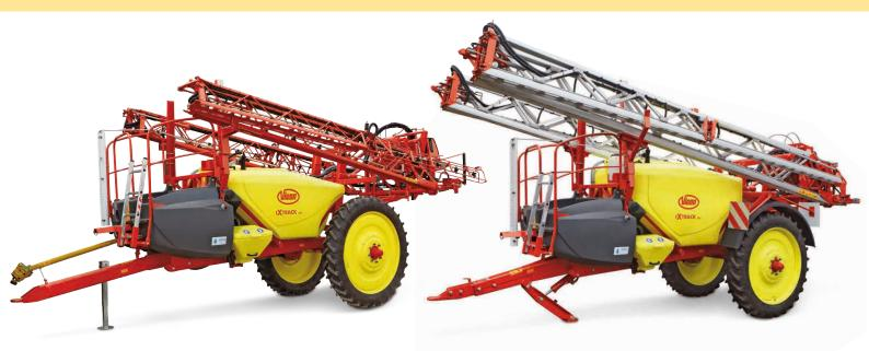
iXtrack A is available in 2400 or 2800 litre tank with HSS 18 up to 30 metre steel booms.
