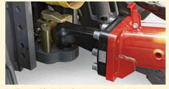
A pulling eye of Ø 40/50mm for low or top linkage or ball coupling Ø 80mm for safe and firm hitching available.
