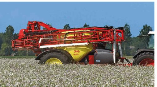
The strong parallelogram system with two lifting cylinders gives an optimum spraying height and no torsion whilst folding the boom in and out.
