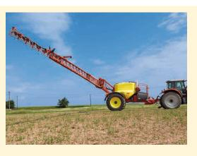
The clever tank design greatly contributes to the sprayers low centre of gravity.
