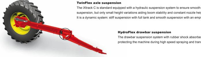
suspension, but only small height variations aiding boom stability and constant nozzle height. It is a dynamic system: stiff suspension with full tank and smooth suspension with an empty tank.
