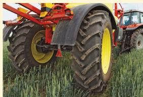
Adjustable suspended axle (iXtrack C30/C40)
