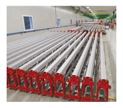
The high tech aluminium boom production location is a closed and ultra clean environment with climate control and pressurisation to guarantee ideal conditions and top quality for the gluing procedure of our famous aluminium booms.
