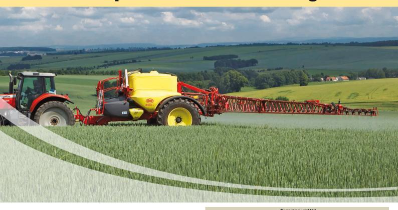
The HSS boom range is designed for professional use. It's triangular construction provides perfect integration of the stainless steel spray lines, nozzles and nozzle holders and the optimal hose routing where all is well protected. The special HSS profile combines a minimum of weight with maximum strength and stability.
