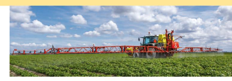
New HC boom designs extends the working widths from 18, 20, 21 and 24m to a more productive 27, 28 and even 30m width. Clever boom folding in symmetrical and asymmetrical patterns gives even greater flexibility for those challenged by smaller fields and in-field obstacles.
