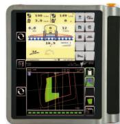
The iXtra operation is integrated in the sprayer's ISOBUS software.
