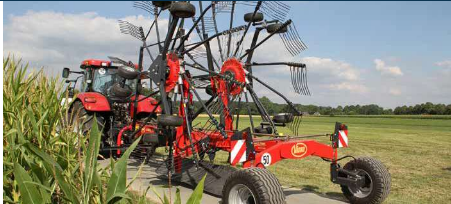
With 9.00m working width and transport height below 4.00m, even without detaching tine arms...
