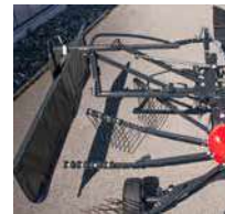
Automatic fold-able swath board with parking stand.
