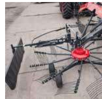
Automatic fold-able swath board with parking stand.
