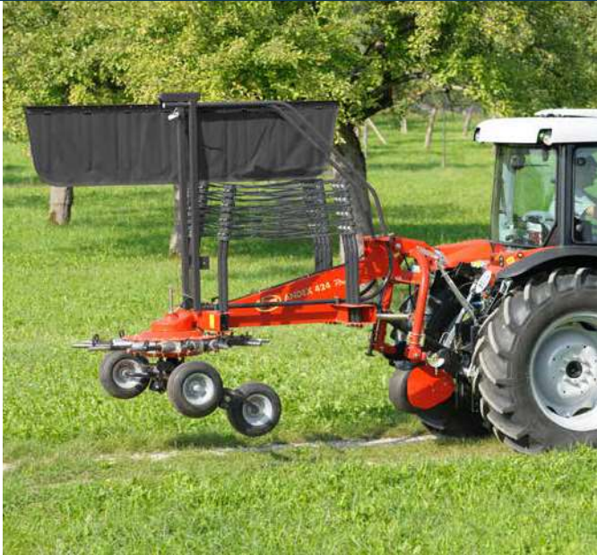
For transport or storage, the rotor guard frames are folded up close to the mainframe, locking automatically into position. An assister spring linked to the swath board reduces the effort required.
