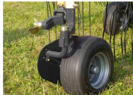
As an option these rakes can be supplied with a third wheel, to ensure even better flotation.
