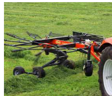
The machine can conveniently be raised up to a height of 50cm from the tractor driver's seat.
