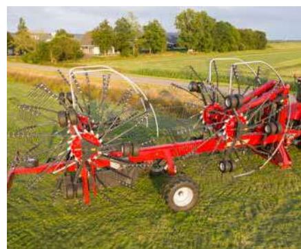
With its' clever folding mechanism the total height remains below 4.00m - despite a rotor diameter of 3.85m. And there is no need to remove tine arms for road transport.
