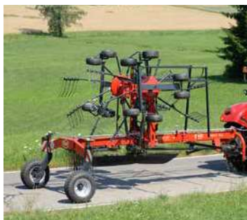
To limit transport height further the tine arms can be removed on the Andex 764. The swath board folds up automatically.
