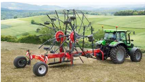
Vicon An dex 1254 Hydraulic lowerable for transport below 4m.
