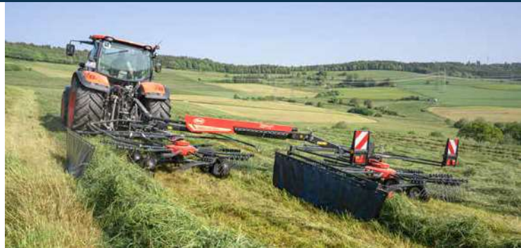
The 715T Vario with 7.10m working width and unique SideShift device.
