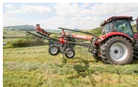
High flexibility on the road, and in the field, as no carrier frame is running on the crop.
