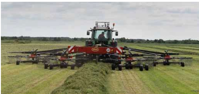
Working width can be set hydraulically between 10-12.5m. Swath width is also set hydraulically between 1.2 and 2.2m.
