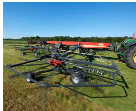
TerraLink Quattro is a unique combination of flexible frame arm and 3-dimensional rotor suspension.
