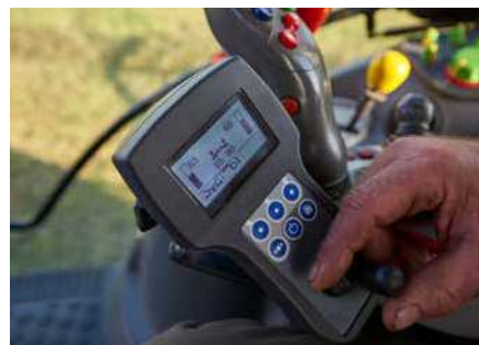
ComfortKit including electronic control of individual rotor height.
