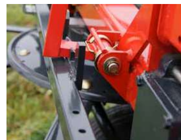
Fanex 464 and Fanex 524 are centrally adjusted for border tedding.
