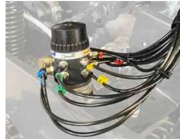
Automatic chain lubrication with individually adjustable outlets.
