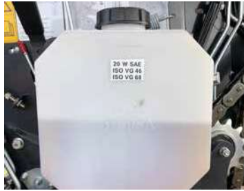
Large capacity chain lube tank.
