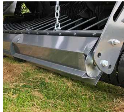
Large diameter roller crop press facilitates crop flow at high intake speeds.
