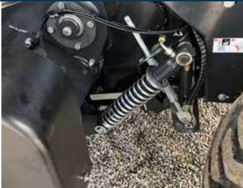
Hydraulic pick-up lift with integrated suspension system for accurate ground following.
