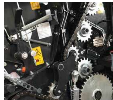
1¼” High specification ‘HBC’ chains are utilised on all bale chamber and rotor drives .
