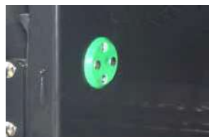
Moisture sensors located inside bale chamber.
