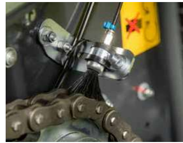
Automatic chain lubrication is standard on FixBale 500.
