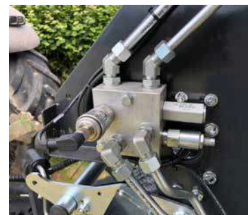
Electronic bale density control.
