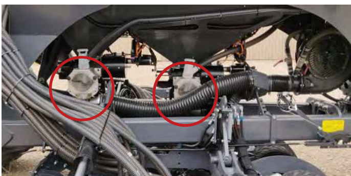
PRO I & PRO II introduced into air circuit of main tank hopper 1 & 2.
