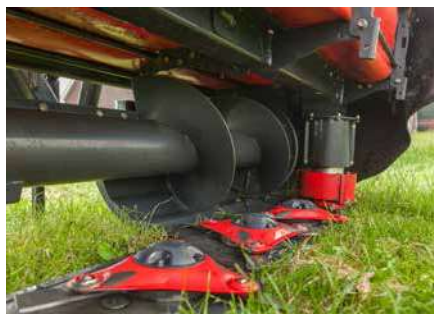
Crop is guided towards the centre by auger and closed guide plates.
