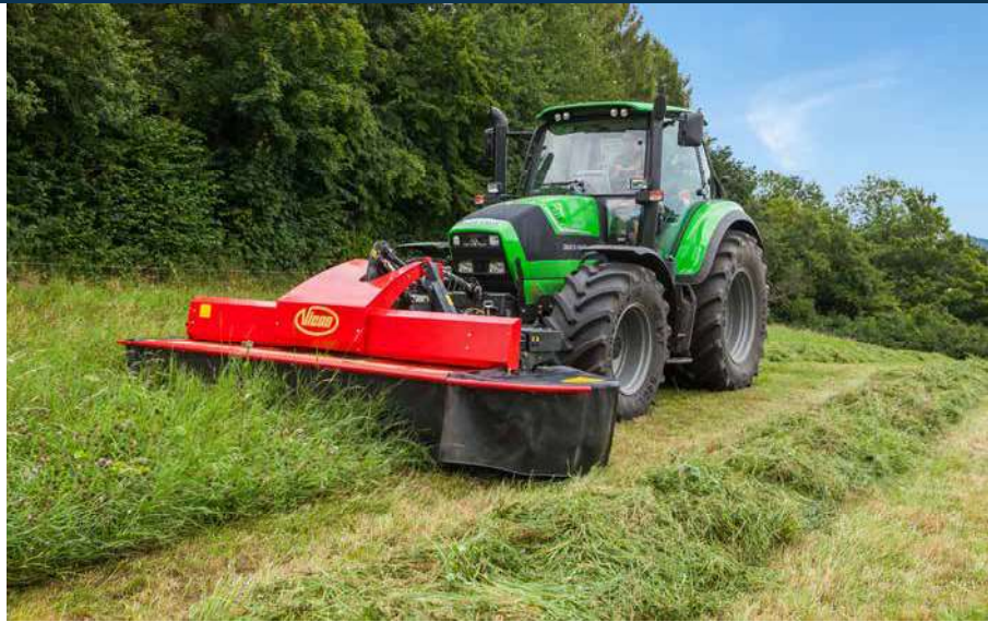
Crop is placed in an airy box shaped swath increasing dry down time.
