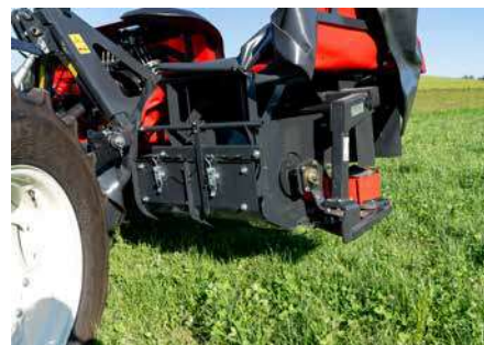
For widespreading the boards are released and positioned on top of the mower.
