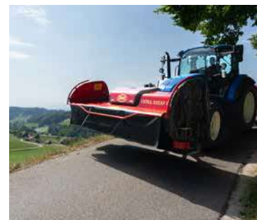
Narrow transport position with good visibility. Hydraulic foldable guards are available as option.
