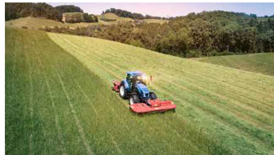
EXTRA 332XF Compact with gravity point close to the tractor is an important feature when operating in hilly conditions with smaller tractors.
