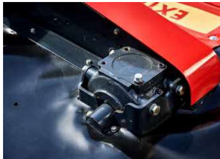
Choice of either clockwise or anti-clockwise driveline, fitting to any tractor supplier.
