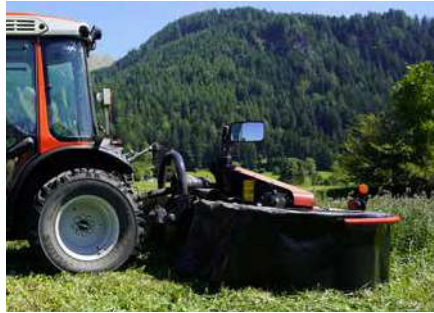
Gravity point is close to tractor for stable, safe operation on steep slopes.
