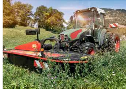
Six or eight counter-rotating discs, each with 3 knives ensure excellent cutting performance.
