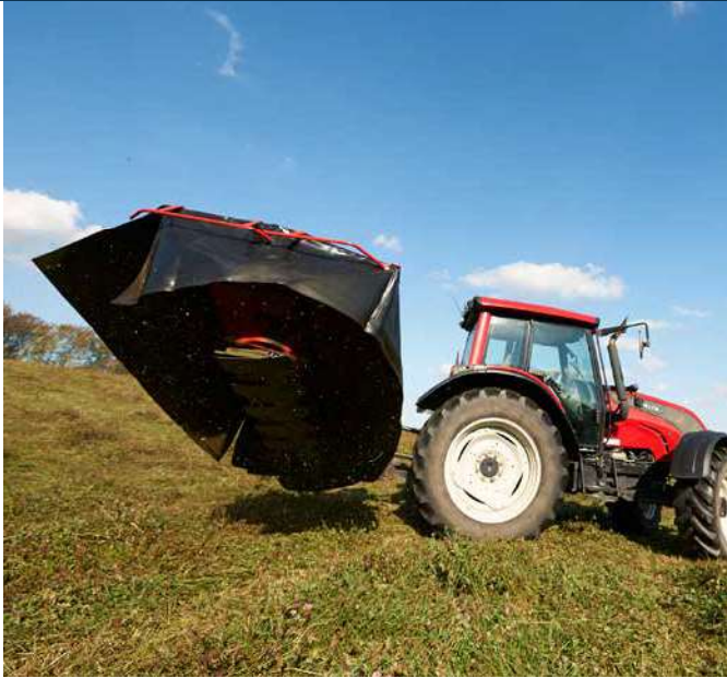
Lifting on headlands via a hydraulic cylinder.
