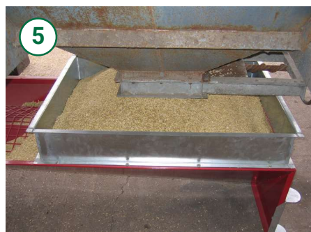
5 An adjustable sluice that controls the flow of grain is required with some of pre-store hopper designs.
