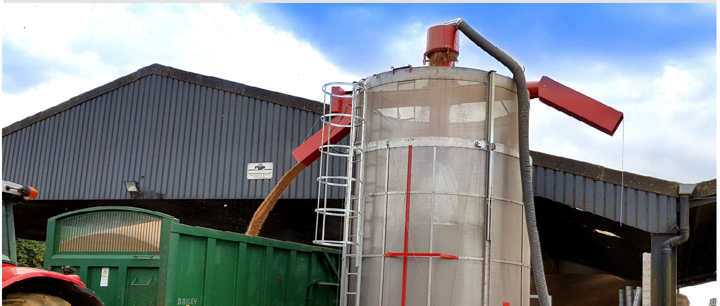
Single: hydraulic or electric horizontal auger to either side
