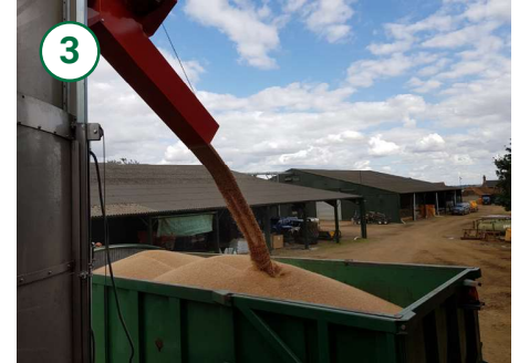
3 Electric or hydraulic horizontal discharge augers can be specified and used to control the speed of emptying.
