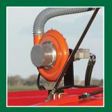
A hydraulic fan provides ample airflow to deliver the granules to the outlets and create a double overlapping spread pattern.
