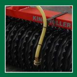
Vertical pipe above the outlet ensures the micro-granules hit the centre of the distribution plate and spread evenly.
