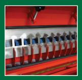
The stainless steel baffle ensures even airflow within the metering system and ensures that only one outlet is fed from each metering segment.
