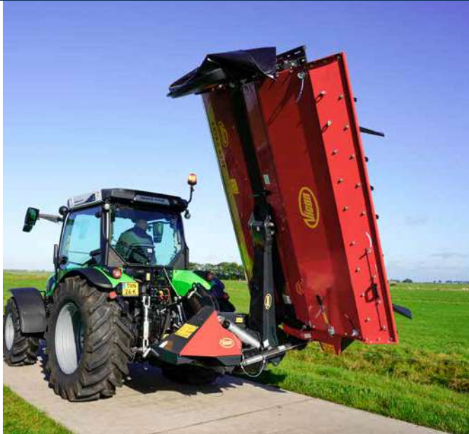
EXTRA 624T, 628T/R and 632T Farmer are folded into vertical transport position using a hydraulic cylinder.
