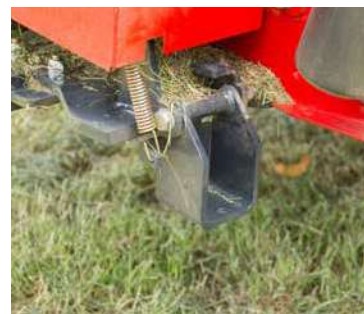
Parking foot is easily activated and keeps the mower in level position when parked.
