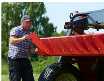
Changing from swathing to widespreading is a one-man job. Simply turn the rear plate 180°.
