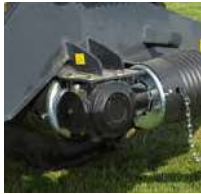
540/1000rpm turnable gearbox as standard.
