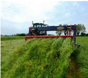
The crop is directed inwards, away from the unmown crop.
