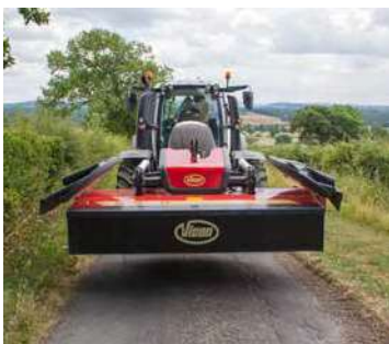
Hydraulic folding of FlexProtect guards (optional).
