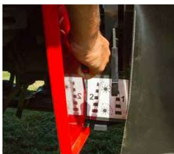
Dual adjustment of conditioner plate to customize to crop intensity.
