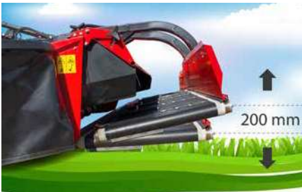
Vicon BX can deliver the crop at different working height.
